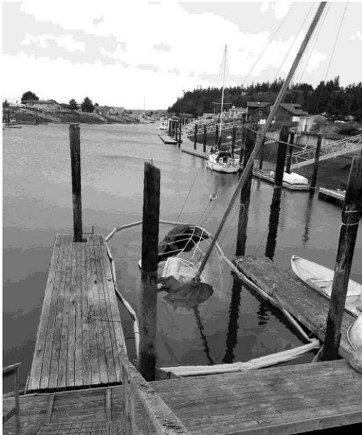
**What caused the boat to sink?** During windy weather in the days preceding the event, the boat's rain cover had been blown open over the aft section of the boat allowing rain to enter the cockpit and run into the bilge. The boat settled just enough that the exhaust thru-hull (with no engine attached) reached the water line. Although a hose was attached to the fitting, the open end had come un-stowed and dropped into the bilge
